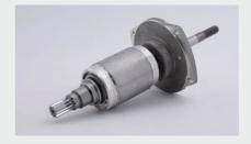
The sliding clutch is located between the motor and the brake so that the power from the brake to the load is transmitted by gear parts in form-fitting connection. Even if the clutch is seriously worn, the load will not fall uncontrolled as the load can be held in every position by the brake.
